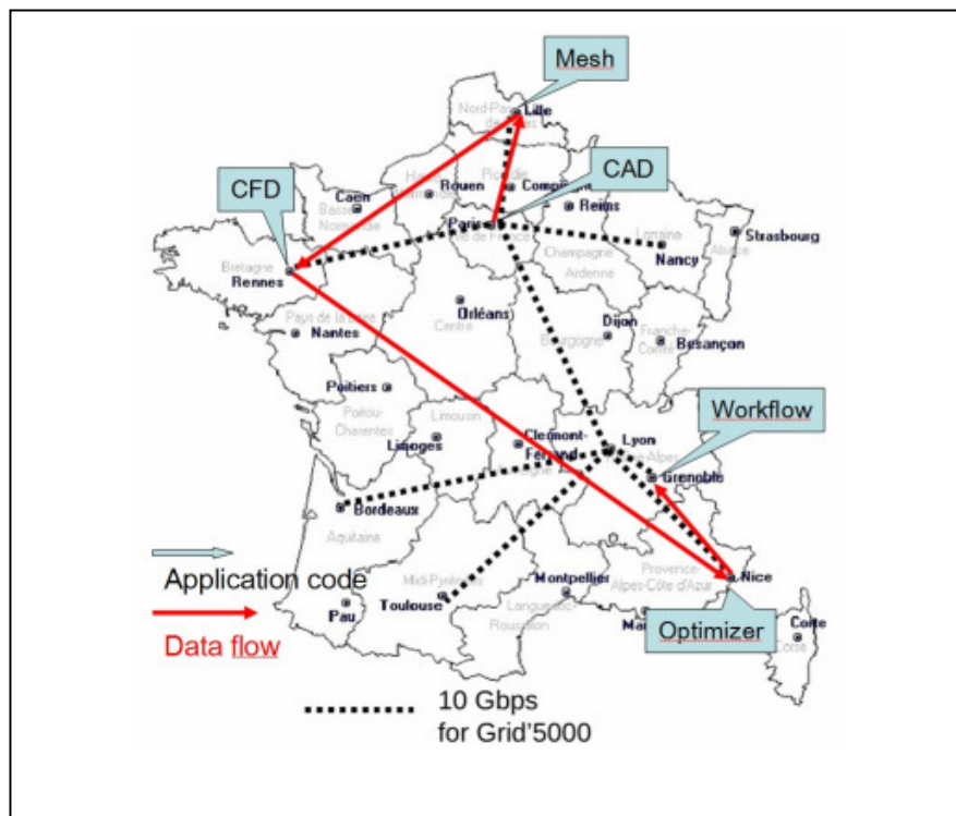
Figure 10. The testcase deployment on the Grid5000 infrastructure.
