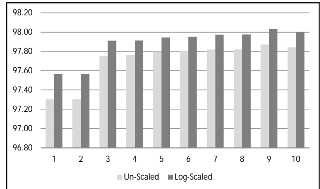
Figure 3: Average classification ratio values from the Cross-Validation, Logarithmic scaling versus unscaled feature space, K = [1,10]
