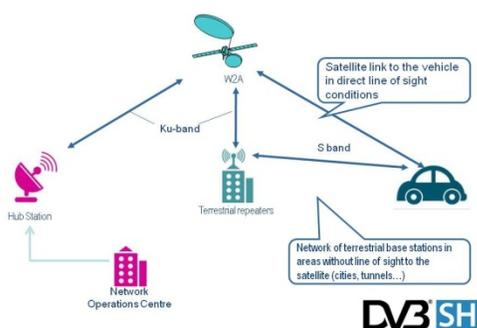
Figure 1. DVB-SH broadcast network architecture
