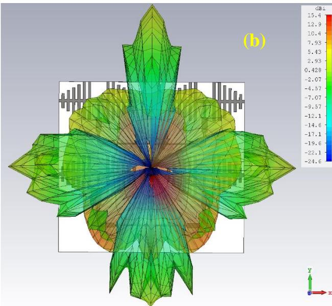
Figure 11. H\_Plan simulated radiation pattern of (2 x 2) antenna array. (a) : 26 GHz, (b) : 27.6 GHz.
