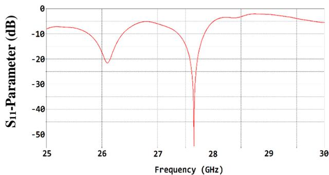
Figure 9. Simulated  $S_{11}$  parameter of (2 x 2) antenna array.
