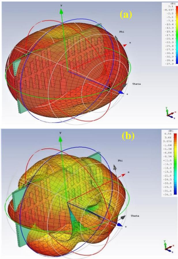
Figure 5. Simulated radiation pattern of elementary antenna. (a) : 3.5 GHz, (b) : 28 GHz.
