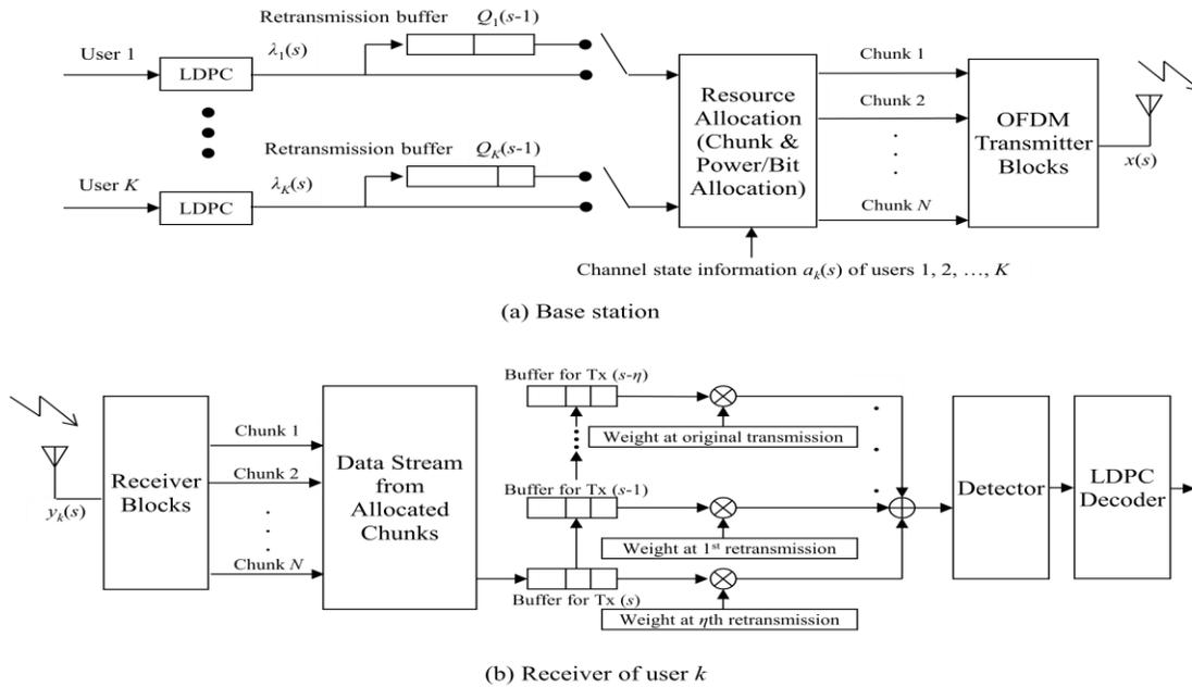
Fig. 1 Downlink multiuser OFDMA block diagram
