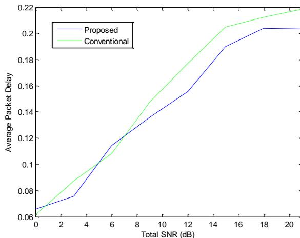
Fig. 3 Average packet delay versus total transmit SNR
