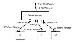
Figure 10. Architecture of triple modular redundancy.
