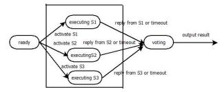
Figure 11. Dynamic behaviour of triple modular redundancy.
