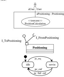
Fig.4. Modelling positioning service
