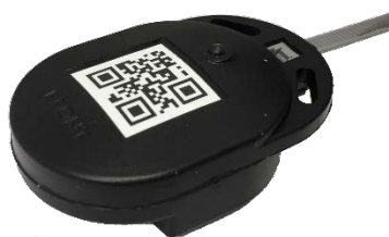
Figure 3. Embedded sensor monitors temperature and relative humidity, calculates strength by ASTM C1074. (Courtesy of ConcreteSensors, http://www.concretesensors.com/products/ ).
