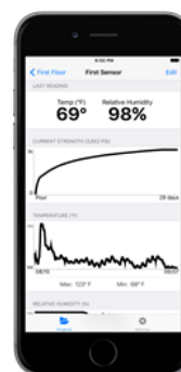
Figure 4. Cellphone interface for embedded maturity sensor. (Courtesy of ConcreteSensors, http://www.concretesensors.com/ )
