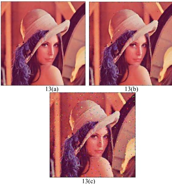
Figure 13. Results by using median filter algorithm for the color image with noise of (a) 10%, (b)20%, (c)30%.
