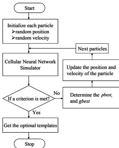
Figure 4. Flow chart of PSO-TVAC-CNN.
