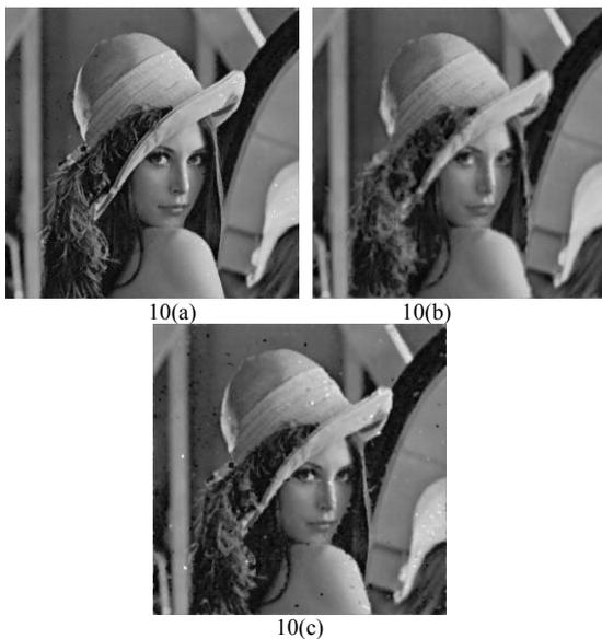
Figure 10. Results by using PSO-CNN algorithm for the Gary-Scale image with noise of (a) 10%, (b) 20%, (c) 30%
