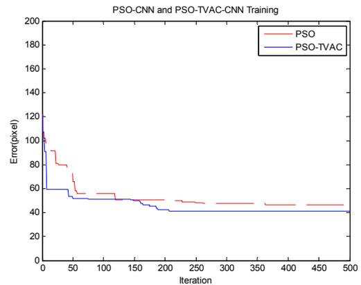
Figure 7. PSO-TVAC-CNN and PSO-CNN Training for Gray image with 20% noise
