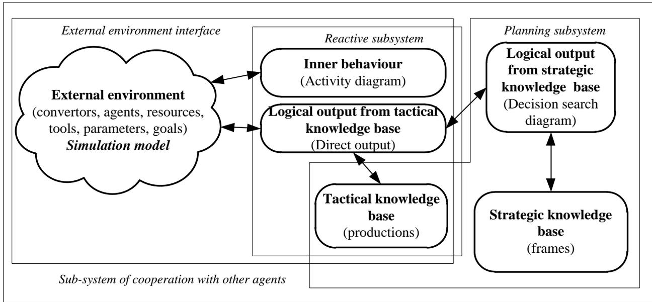
Figure 1. Multi-agent resource conversion process model structure
