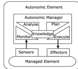
Figure 1. MAPE-K intelligent control loop [8, p. 6]
