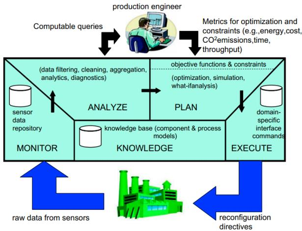
Figure 2. MAPE-K applied to smart manufacturing [9, p. 5]
