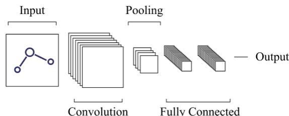
Figure 2. Diagram of a simple five-layered CNN architecture.
