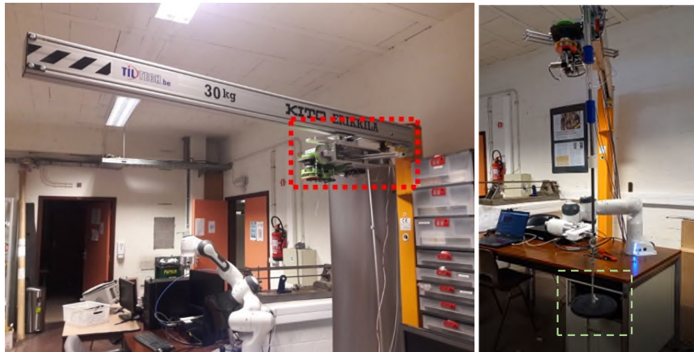
Figure 5. Jib crane with a gravity compensator (left – red dash line) coupled to a Franka Emika Panda Cobot (right). The payload of the cobot is initially 3kg (the gripper weighting already 0,8kg) and the manipulated load (black cylinder – green dash line) weighs 5kg
