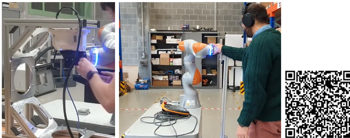
Figure 8. (Left) AMR in a 3 rd hand configuration, (Middle) AMR in Joystick configuration, (Right) QR code of a video with the 2 realizations
