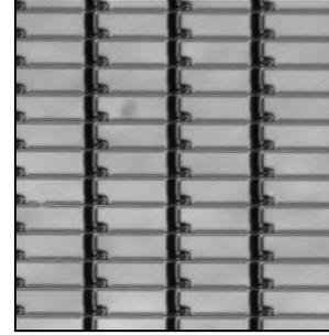
Figure 1. The image of a TFT-LCD panel under the fine resolution of 120 pixels/mm.
