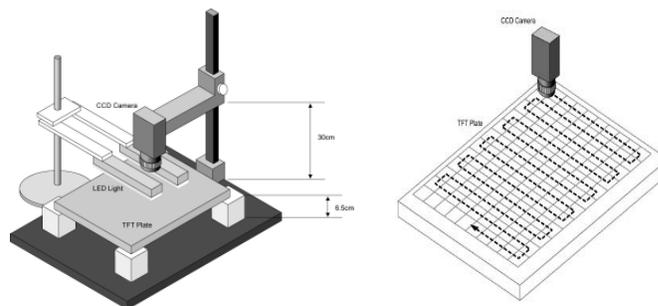
Figure 6. The configuration of the automated LCD inspection system, and the scan trajectory of the camera.
