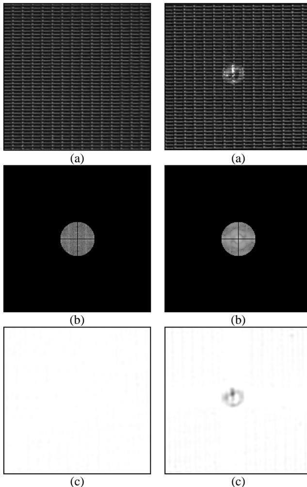
Figure 4. (a) The same faultless TFT- LCD sample shown in Figure 2(a); (b) the corresponding power spectrum, in which the black regions represent  $F(u, v)$  with a set value of zero; (c) the reconstructed image from (b).
