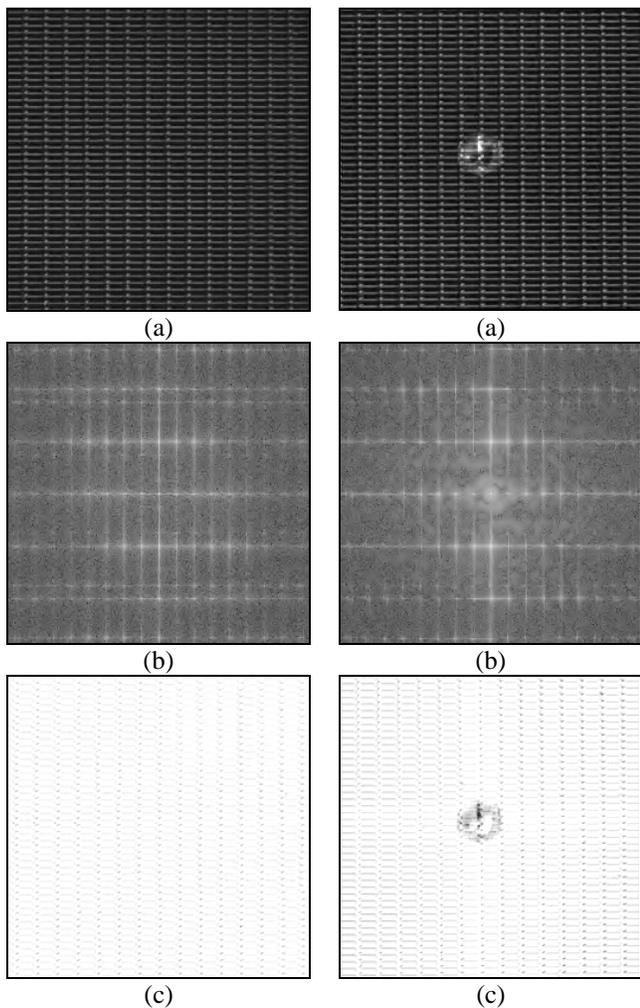
Figure 2. (a) A faultless TFT-LCD surface; (b) the corresponding Fourier power spectrum; (c) the reconstructed image by setting
