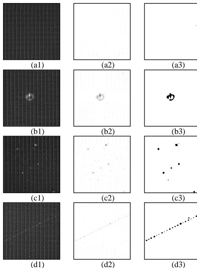
Figure 7. Four TFT-LCD panel images used for test: (a1) a faultless TFT-LCD surface; (b1)-(d1) defective TFT-LCD surfaces with respective pinhole, particle and scratch defects; (a2)-(d2) reconstructed images; (a3)-(d3) resulting binary images.
