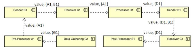
Figure 3. Execution path using the dynamic management
