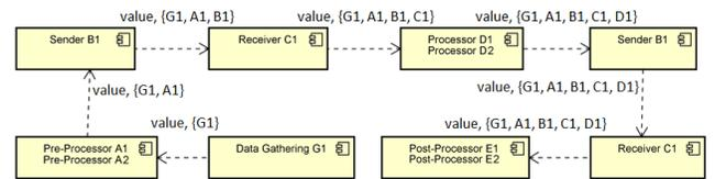
Figure 2. Execution path of the data in a partially reconfigured system
