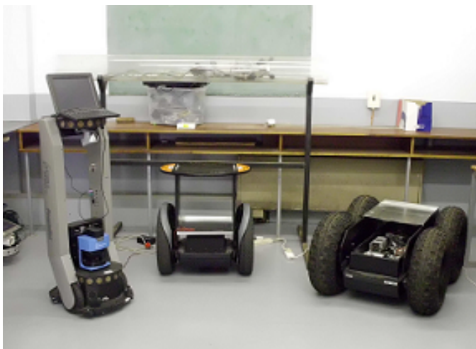
Figure 3. Mobile robot hardware used for the research
