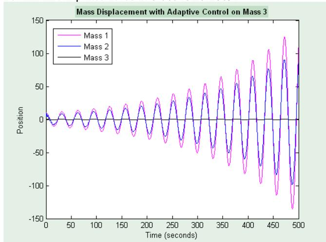
Figure 4. Adaptive key component controller on mass 3.
