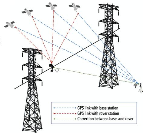
Figure 6. Scheme of global localization through RTK GNSS.
