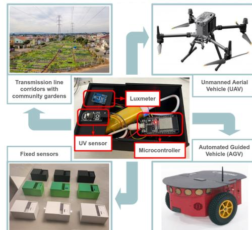
Figure 1. Project workflow and development of the measurement system using fixed and mobile robotic platforms.
