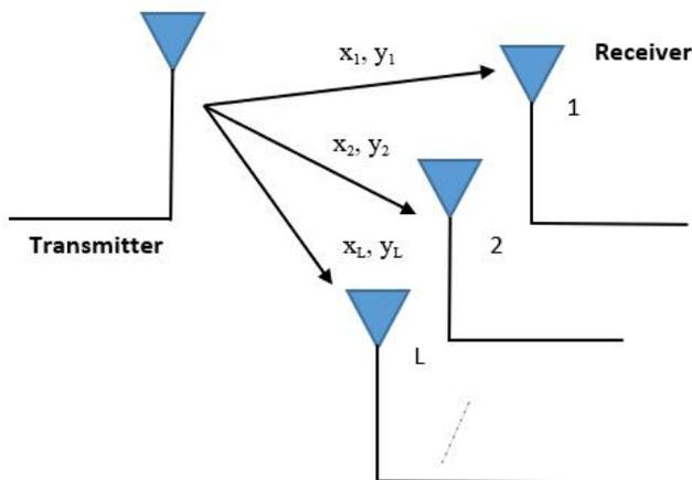
Figure 1. Model of a selection combining diversity receiver.
