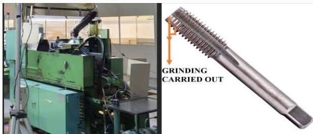
Figure 3. RD6 Machine and Rectified chamfered piece.
