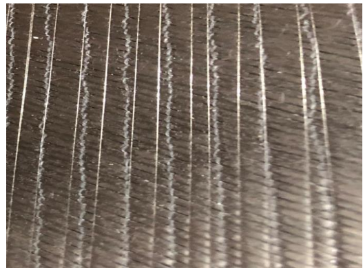
Figure 1. Image of the carbon fiber composite with magnetic microwire inclusions (the vertical lighter fibres) with 5 mm spacing.
