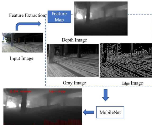
Figure 1. The process of obstacle detection
