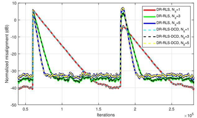
Figure 1. Performance of the DR-RLS and DR-RLS-DCD algorithms for different values of  $N_{it}$ . The unknown system changes at time index 60001, and the SNR is decreased for 5000 iterations, starting with index 180001.
