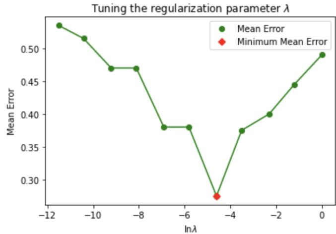
Figure 2. Tuning the multilayer perceptrons through 10-Fold Cross-Validation for choosing the regularization parameter  $\lambda$  according to the elbow rule. The minimum mean error is achieved when  $\lambda = 10^{-2}$
