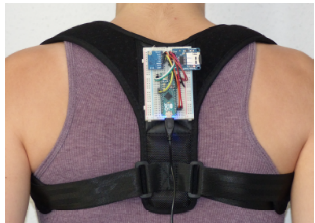
Figure 1. Wearable sensor platform fixed at a test subject's upper body.
