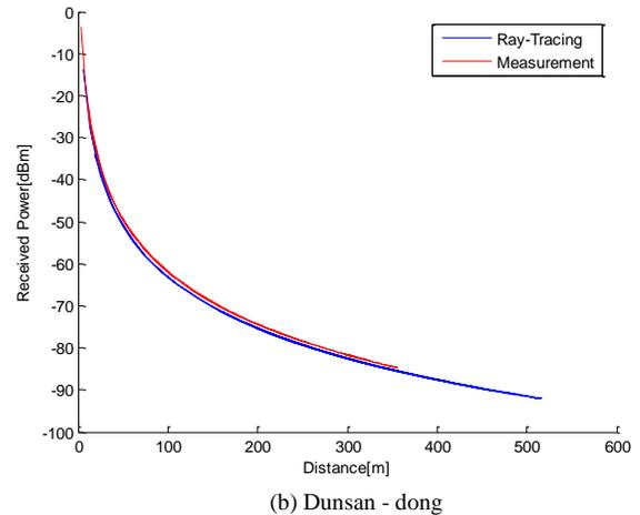
Figure 6. Comparison between Ray-Tracing and measurement
