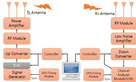
Figure 2. Measurement system configuration
