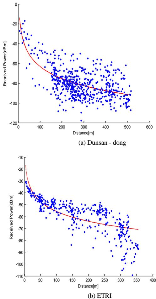
Figure 3. Received level of our measured data
