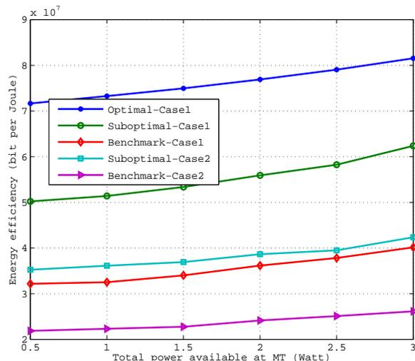
Figure 2. Average achieved energy efficiency versus total power available at each MT [42].
