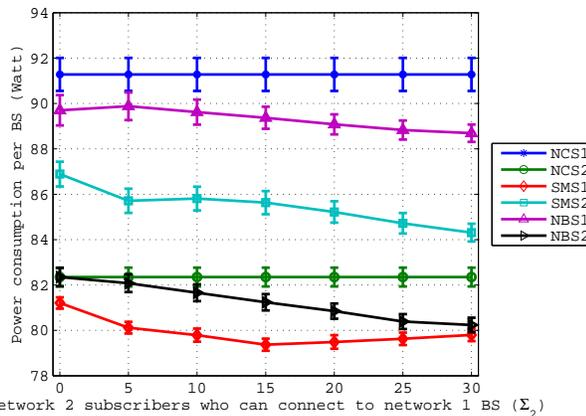
Figure 3. Power consumption for each BS versus the number of network 2 subscribers who can connect to the BSs of both networks [43].
