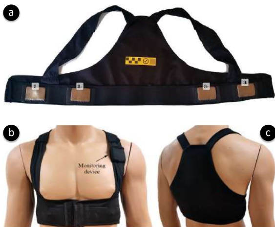
Figure 2: Textrode Sensorized Vest;(a) electrode placement in the inner side view (b) front view and monitoring device, (c) back view.
