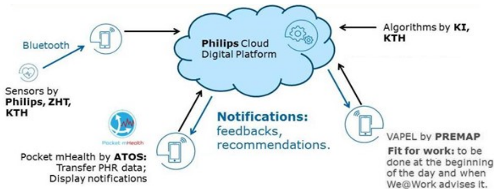
Figure 3: We@Work Architecture Framework
