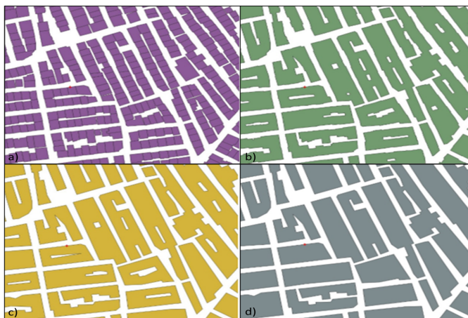
Figure 3. Illustration of used GIS operations to buildings' polygon data quality improvements and their results for the sample dataset. (a) Original data, (b) the aggregated polygons, (c) simplified polygons, and (d) deleted holes from the buildings' polygon.
