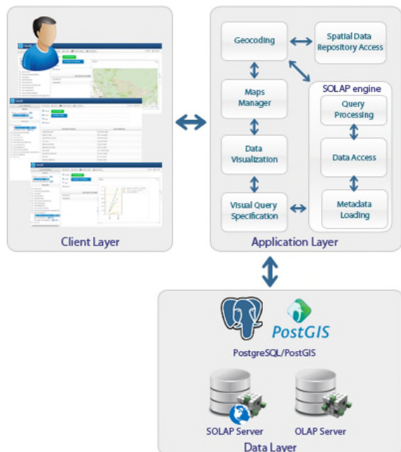
Figure 1. The SOLAP_Frame architecture.
