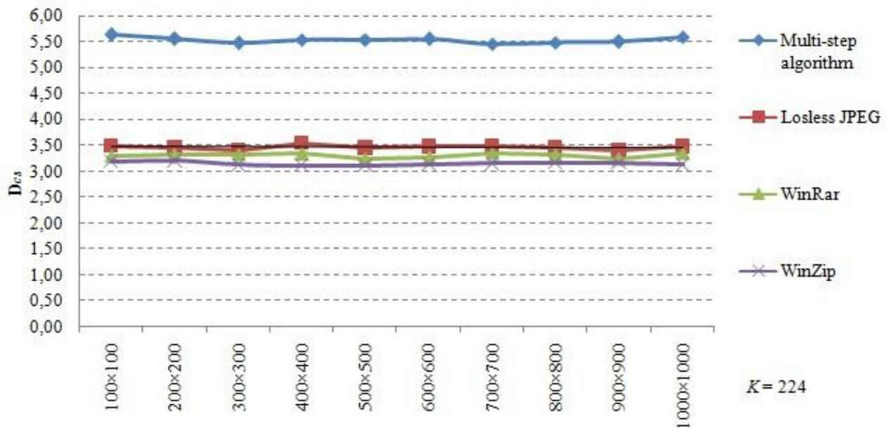
Figure 3. Comparative effectiveness of compression algorithms for different geometrical size of scene.
