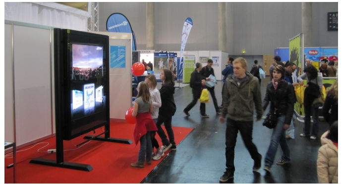
Figure 2. Setup of large-scale public display at Vienna Sports World Fair. Depth cameras were used to detect and extract behavior features for effort computation.
