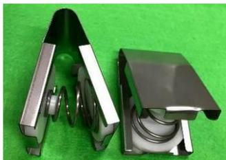
Figure 7. Two views of the simple heel-raising unit.
