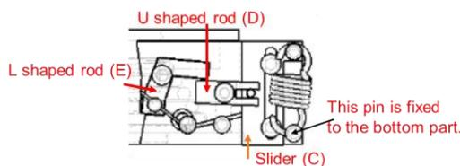
Figure 9. Structure of the release timing control part
