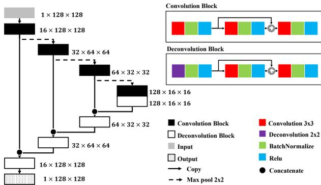
Figure 2. The convolution neural network for the eye-frontalization.
