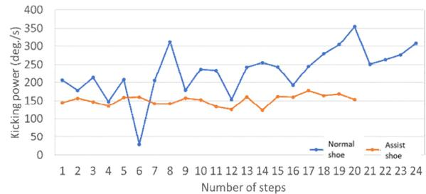
Figure 7. Kicking power when heel is raised with normal and proposed assist shoes for a stroke patient.
