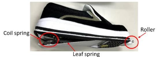
Figure 6. Assist shoe prototype.
