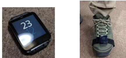
(a) WD: SmartWatch 3, Sony (b) WD mounted on foot
