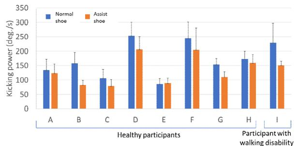
Figure 8. Kicking power when heel is raised with normal and proposed assist shoes.
