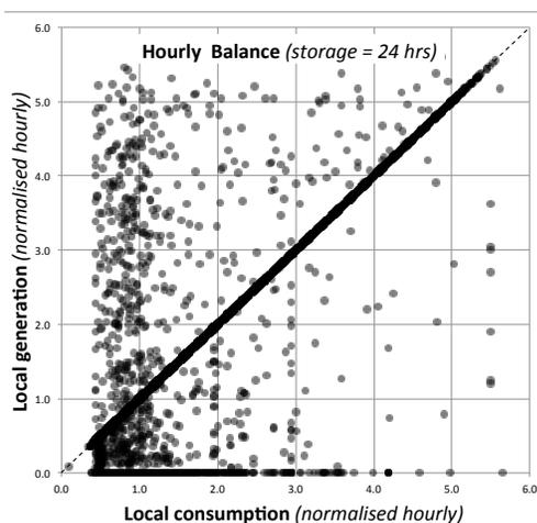
Figure 2. Energy balance at hourly intervals over a year for an example installation.
