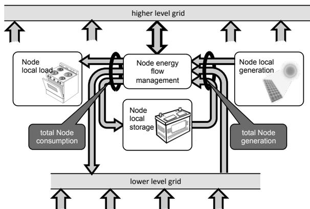
Figure 4. A fractal microgrid energy flow model.
