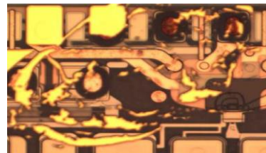
(a) Gold resist in various stages of damage
