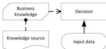
Figure 1. DRD-level elements
