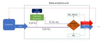
Fig. 7. Feature selection and decision making procedure in more details for the second solution.
