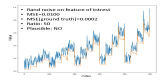
Fig. 13. Testing agent for predicting feature-1 based on 3 most related feature. Random noise on the FoI, MSE =0.01 (50 times higher than the ground truth). (Blue: real data, Orange: predicted data)
