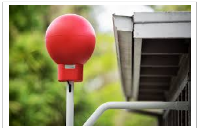
Figure 5. Project Loon Signal Receiver
