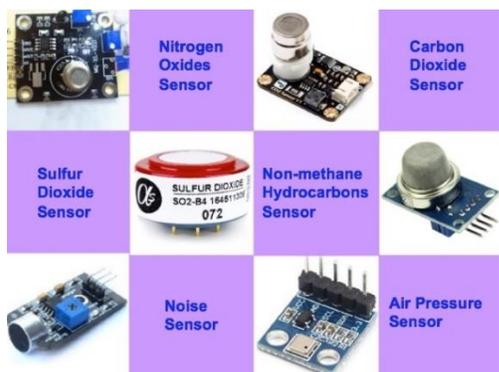
Figure 7. Exemplar Components aboard 3DP Sensors
