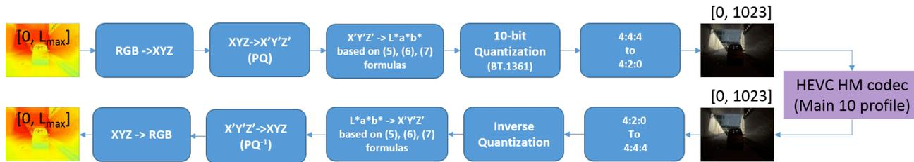
Figure 3. Pre/post processing steps of the proposed modified CIELAB for HDR video compression
