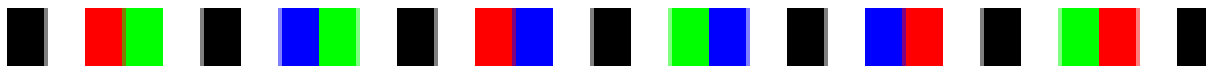
Figure 1. Structure Light Pattern containing 6 unique color edges. Total number of edges to be extracted from one 2D image is 32
