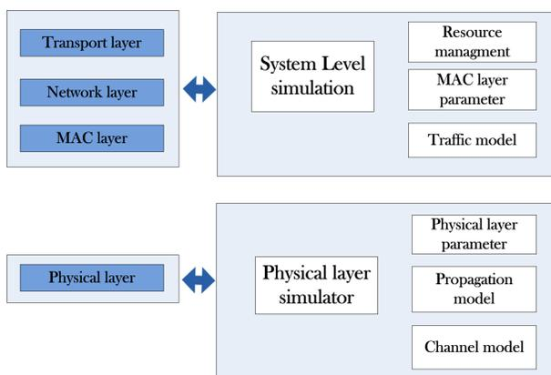
Figure 7. Component layers and model for simulation methodology [2]
