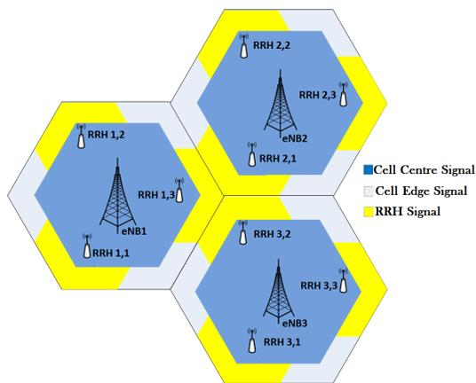
Figure 6. CoMP deploying RRH antennas
