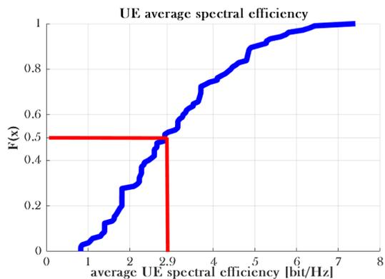
Figure 14. UE Average spectral efficiency (bit/Hz) versus F(x)
