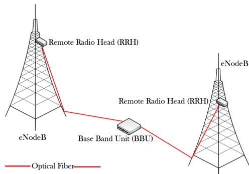
Figure 1. Remote Radio Head (RRH) Deployment
