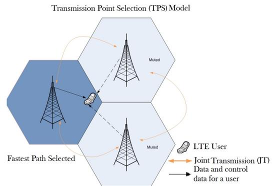
Figure 5. Transmission Point Selection (TPS)
