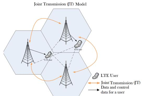
Figure 4. Joint Transmission (JT)
