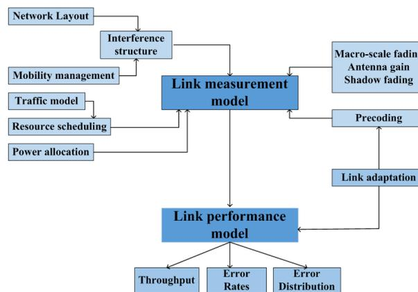
Figure 8. Schematic block diagram of LTE-A SL Simulator [12]
