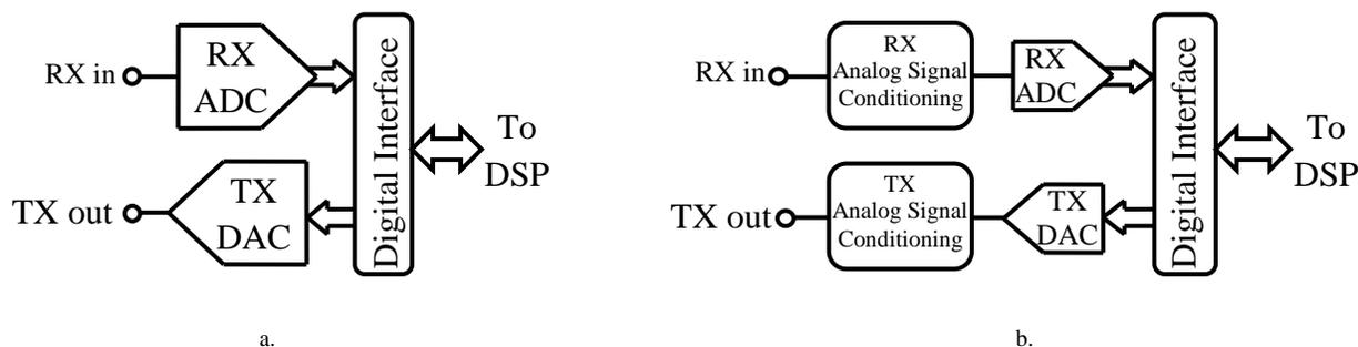
Figure 3. Software Defined Radio Simplified Block Schematic (FS and AUX not shown):
