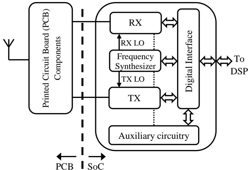
Figure 2. Software Defined Radio Transceiver Generic Block Schematic.
