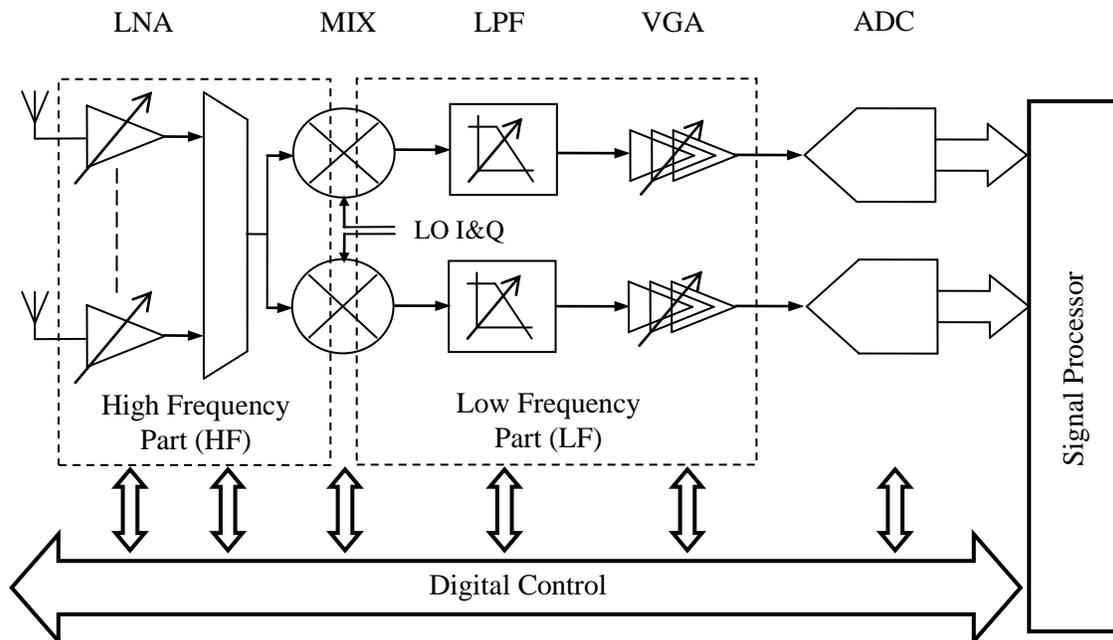
Figure 4. Software Defined Radio Transceiver Block Schematic [6].
