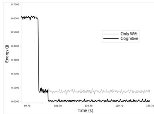
Figure 4. Power consumption for the Cognitive algorithm and WiFi
