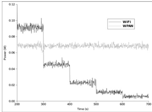
Figure 6. Power consumption for the Cognitive algorithm and WiFi (Scenario 2)
