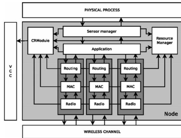
Figure 1. Castalia node internals adapted to cognitive radio
