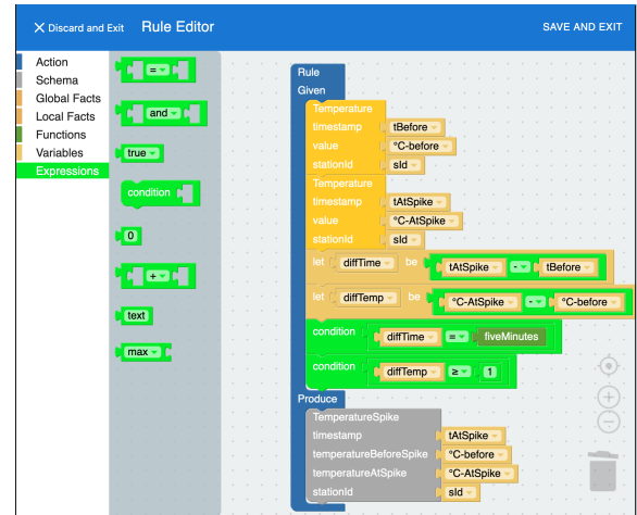
Figure 6: Screenshot of the visual editor for rules to detect temperature spikes.
