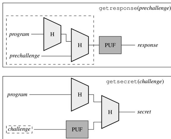
Figure 2. Algorithms to access the CPUF [17].
