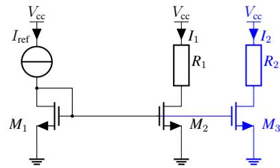
Figure 3. Current mirror as a constant current source.
