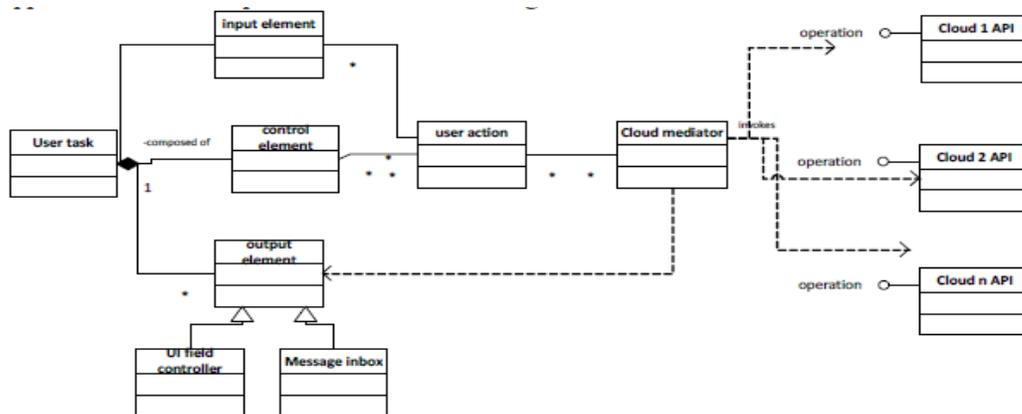
Figure 1: Architecture of mediator-based virtualization of cloud services
