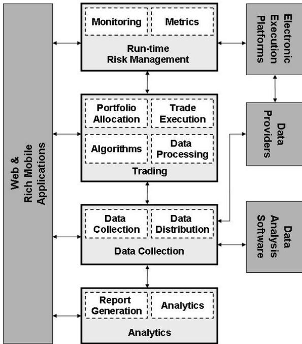
Figure 1. Reference component architecture of a contemporary on-premise high-frequency trading platform.
